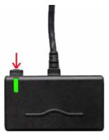
3. When the indicator on signal receiver is flashing, use the signal pen to press the "Code" button on the tablet back. Following Add Tablet window appears.
